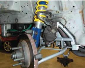
PN 20110) until the spring is compressed to achieve ride height. Once the spring is loaded push the key into its groove and tighten the 10-24 button head screw. The adjustment of the nut allows for changes in ride height and may need to be tuned to you desired needs.
